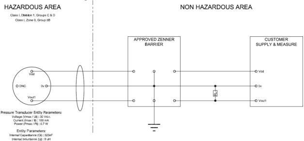
**Absolute Output Mode:** (Typical output ranges are 0-10V, 0-5V, 1-6V and 1-5V)
